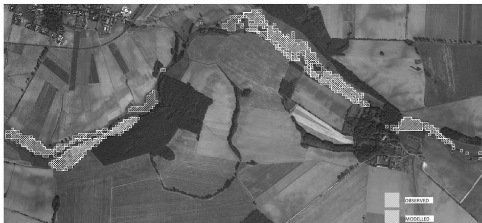
**Fig. 3.** Observed and modeled flood extents
