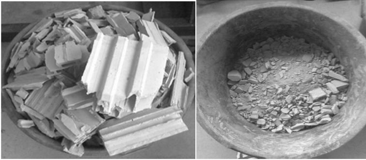
**Fig. 1.** Ceramic waste and ground ceramic waste
