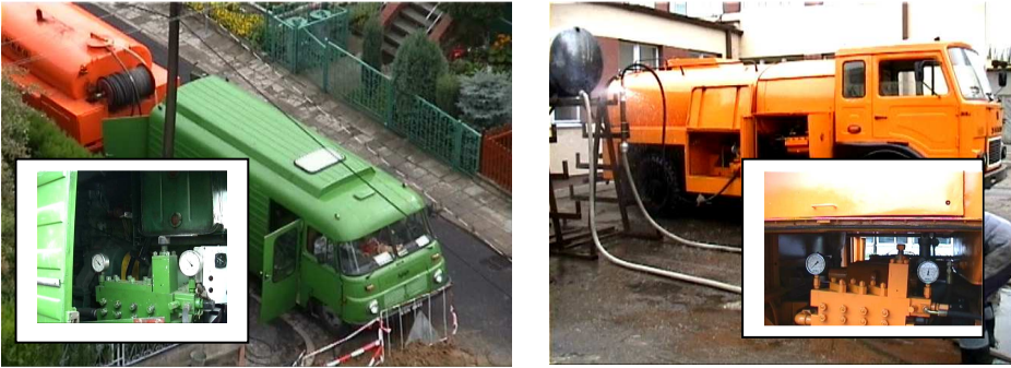
Fig. 8. General view of two mobile test stands based on a hydro monitor with a highpressure pump
