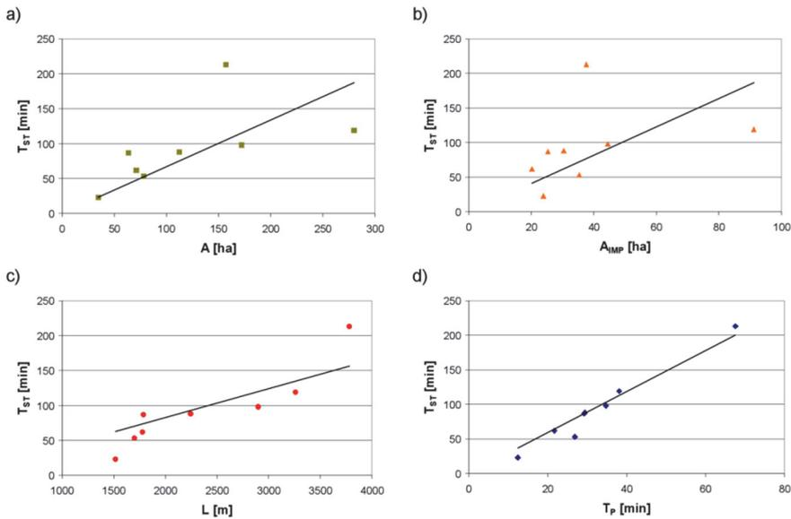
**Fig. 4.** The results of the analysis of the correlation between the catchment characteristics and the stabilization time  $T_{ST}$
