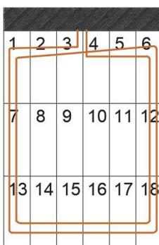
**Fig. 4.** Division of the power pad into sectors
