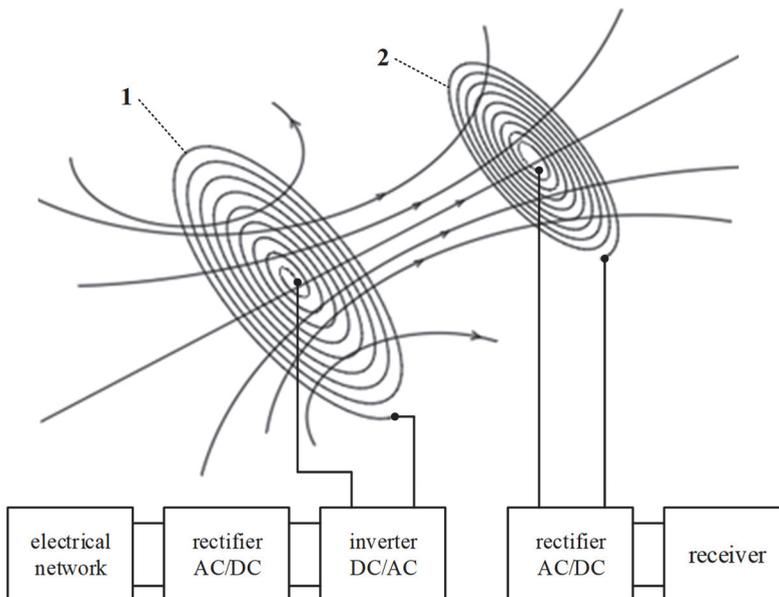
**Fig. 2.** Block diagram of the system for wireless energy transmission:
