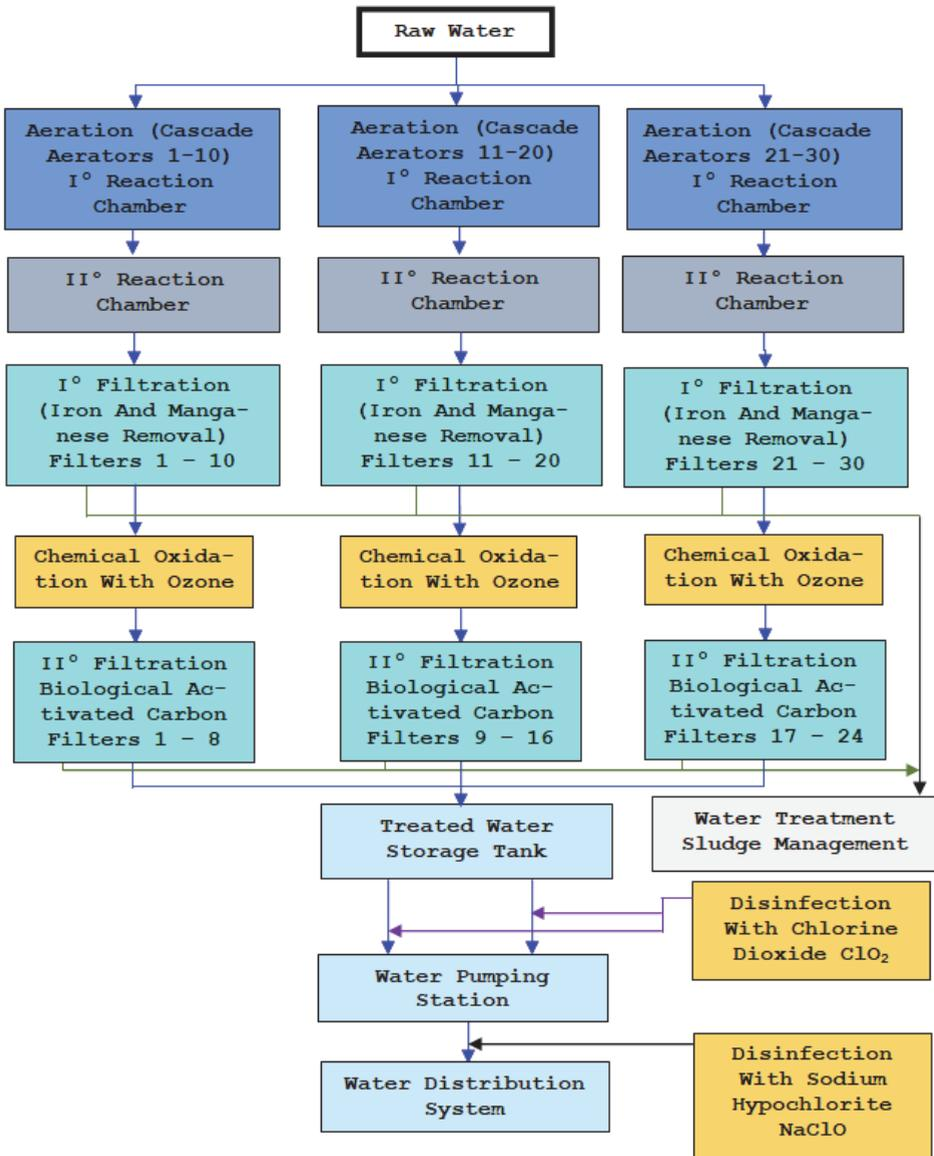
Fig. 1. The scheme of the Water Treatment Plant
