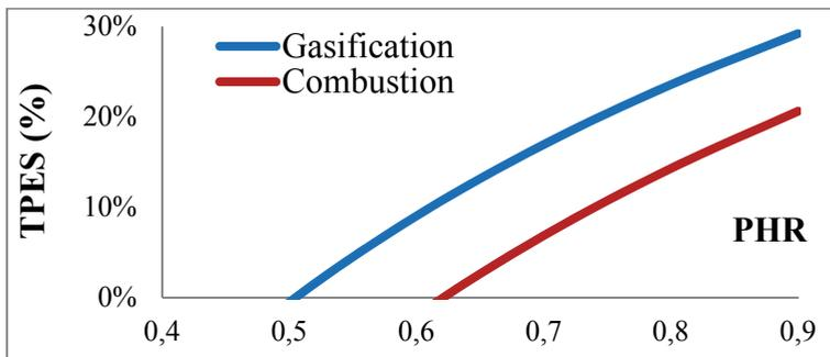
**Fig. 4.** Trigenation primary energy saving depending on Power to Heat Ratio
