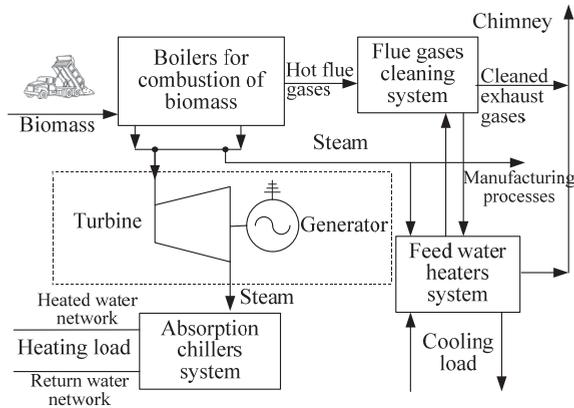
**Fig. 2.** Exemplary diagram showing the biomass combustion in a trigeneration system
