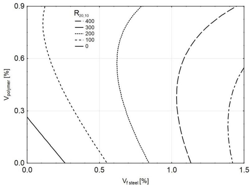
**Fig.7.** Residual flexural strength factor  $R_{20,10}$
